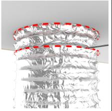
Cut off excess flexi duct 2 ribs below ceiling level.
