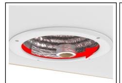
Attach flexi shaft to inside of ceiling ring collar with aluminium tape provided.
