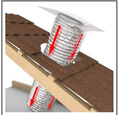
Drop flexi shaft through the opening in the roof sheeting.
