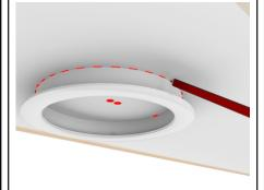
From ground level (looking up at ceiling) locate the original hole for positioning ceiling ring. Hold ceiling ring to ceiling with hole in dead centre. Trace the outside of the collar with a marker.
