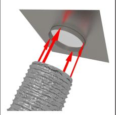
Slip the flexi shaft over the metal collar on the underside of the skylight dome.
