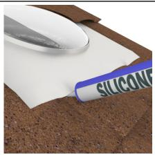
Use silicone to seal under edges of tray to roof sheeting.
